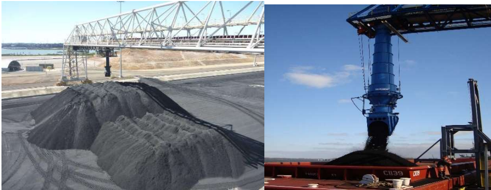
Figure 47. Telescopic Chute to Minimize Freefall of Aggregates (PEBCO, 2020)
