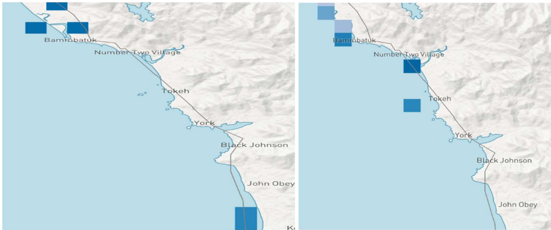
Figure 39. Flood Inundation Model Output for Black Johnson up to 2030 (Left) and 2080 (Right)
